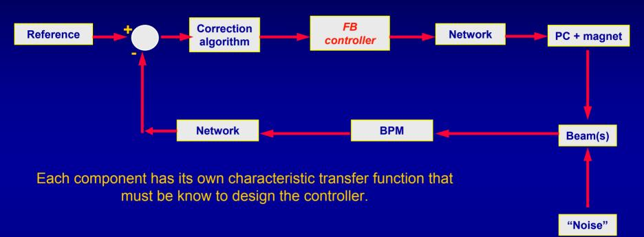
This RT loop spans the entire LHC machine. For good performance :
